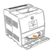
To load envelopes that are under 8.66 inches (220 mm) in width, insert the envelopes with the flaps open and toward the front of the printer, with the recommended print side face up.
