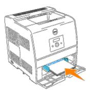
4. Slide the width guides until they rest lightly against the edge of the print media stack.
