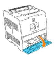
2. Slide the width guides to the edge of the tray. The width guides should be fully extended.
