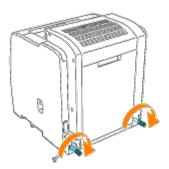
7. Open the optional duplex module. Remove the connector cover, and then attach the connector on the bottom left of the optional duplex module to the printer. Keep the original cover somewhere safe.
